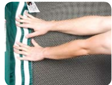
Fig. 45A. ALWAYS test that the zipper is securely closed by pressing against the entire length of the closed zipper to make sure it will not open when pressure is applied
