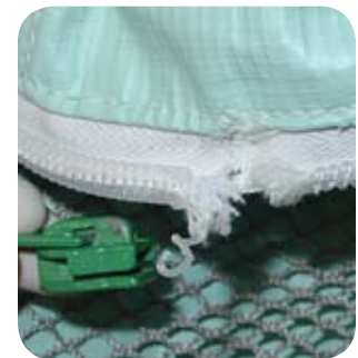
Fig. 43. Zipper Teeth Broken
